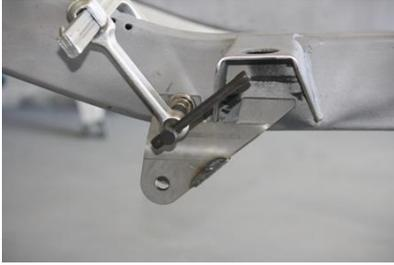
**STEP 5:** Once installed, recommend installing leaf springs and shackles to check fit. Once satisfied, weld front and rear mounts to the frame.
