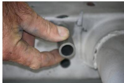
**STEP 2:** Install 7/8" DOM sleeve into hole on driver and passenger side of frame. Note: Hole may need to be cleaned out slightly for spacer to fit.
