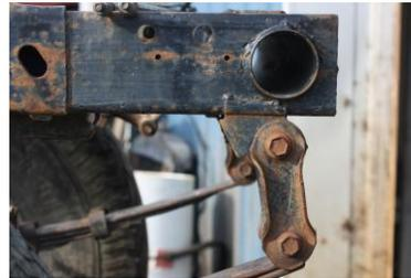
**SUGGESTIONS:** Grind or torch off mounts. Use a cutoff wheel to cut welds without cutting into frame. Mounts can then be removed from the frame.
