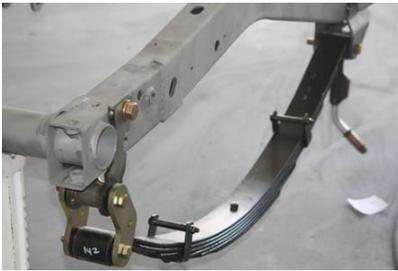
**STEP 6:** Once welded, clean up and paint and reinstall axle, shocks, u-bolts, etc. and torque to factory specs.
