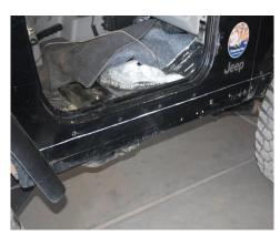
Measure 2" in from outside of body on the bottom side of the floor. Make your line. Once everything is measured out and lines are drawn, you can begin your cuts. A plasma cutter works the easiest but you can use a cut off wheel, jigsaw,OR sawzall. Note: Before you make your cuts, make sure everything is moved out of the way on the inside of the jeep.
