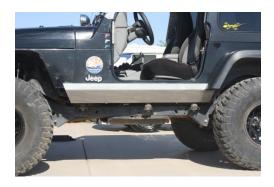
Once holes are drilled, boat sides can be bolted up. When you are happy with the fit, boat sides can be removed and painted or powdercoated, then reinstalled for good.
