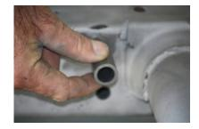
**STEP 2:** Install 7/8" DOM sleeve into hole on driver and passenger side of frame. Note: Hole may need to be cleaned out slightly for spacer to fit.
