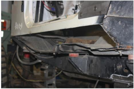
Once you have cut and removed the rocker section, clean up the edges with a grinder and touch up any bare metal with paint or undercoating. Loosen side body mount bolts. Note: Boatside will be sandwiched between floor and center body mount! Clamp boat sides up against body. Once you are happy with the positioning, the outside holes can be drilled. You will need to use a 3/8" drill bit. Note: Access holes may need to be made on the inside of the body because of a double wall to install the nuts.
